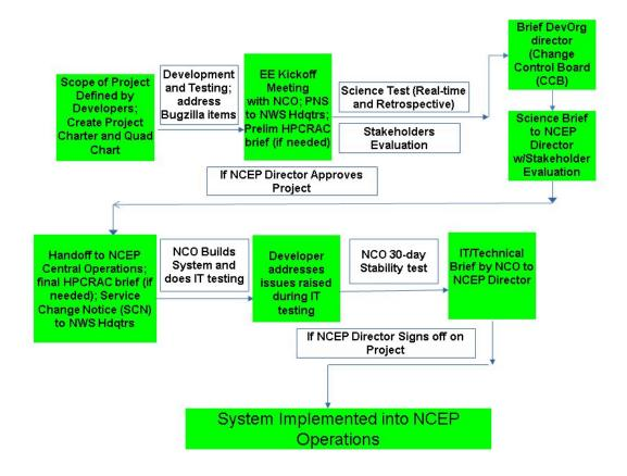
Figure 1: NCEP Implementation Process : Flowchart
