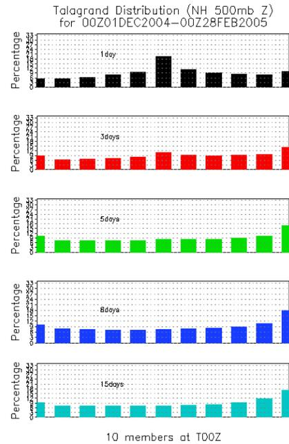
Figure 2 shows an example of a NCEP GEFS (10-member) forecast for the period December 1<sup>st</sup> 2004 – February 28<sup>th</sup> 2005, for 1-, 3-, 5-, 8-, and 10-day NH 500hPa geopotential height. The histogram distribution for the raw forecast is over-dispersed at the short lead-time at that time period. There is a little cold bias for longer lead-times as you see the high bars move right as lead time increases.
