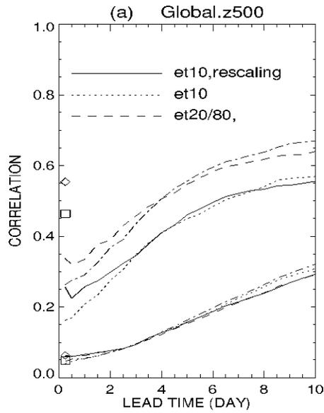
Fig. 3. PECA values for a 10-member ETR (solid), 10-member ET without rescaling (dotted), 20 of 80 member ET with rescaling (dashed) and 20 of 80 member ET without rescaling (dash-dotted) ensembles for (a) the globe; (b) Northern Hemisphere; (c) Southern Hemisphere and (d) the tropics. Shown in thick and thin lines are PECA from the optimally combined perturbations and average PECA from individual perturbations, respectively.
