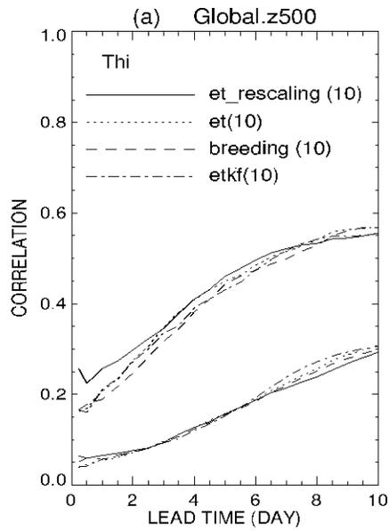
Fig. 2. PECA values for ETR (solid), ET without rescaling (dotted), breeding (dashed) and ETKF (dash-dotted) ensembles with 10 members for (a) the globe; (b) Northern Hemisphere; (c) Southern Hemisphere and (d) the tropics. Shown in thick and thin lines are PECA from the optimally combined perturbations and average PECA from the individual perturbations, respectively.
