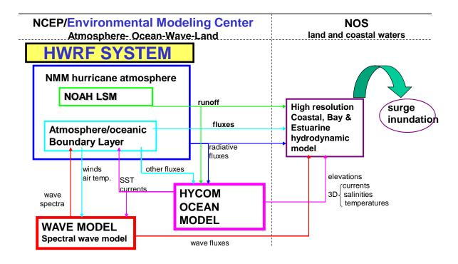
Figure I.2. Proposed future operational coupled hurricane forecast system.
